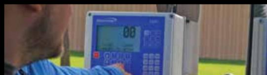
Driver approaches the LS20 Indicator, stops and keys in the Truck ID, or activates the system with the optional Key Fob. Driver proceeds over the scale and visually receives a weight on an LED display, with a red/green stop and go light. All weight data is collected for download onto a USB or serial connection.
